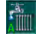
Automatic mode (automatic switch between working modes Heating+DHW and only DHW mode)
